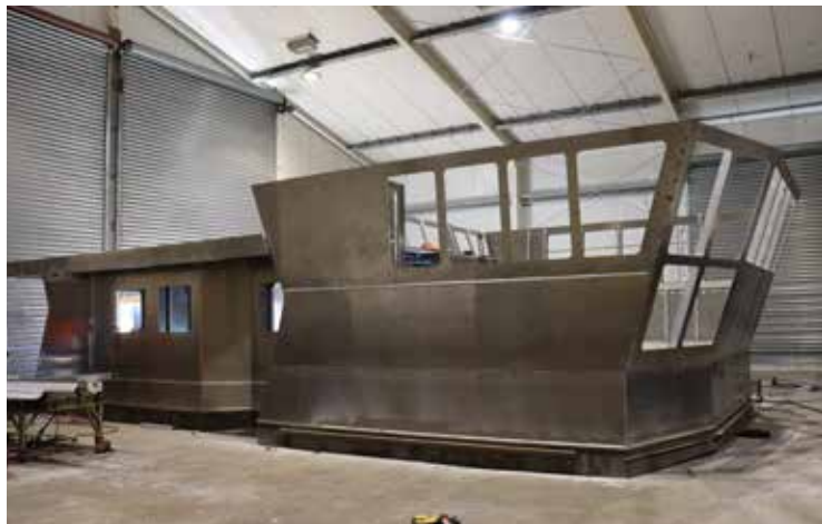
The wheelhouse of Westfleet's $6m trawler Te Runanga under construction at Aimex.
