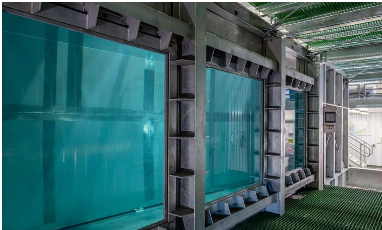
The largest tank of its type in New Zealand – the 190,000 litre flume can get the water moving up to 1.5 metres per second.
